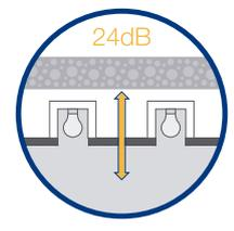
Ceiling with downlighters treated with Acoustic Hoods ( $R_w$ )
