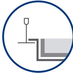
Soundblocker in a perforated metal tile with the foam facing downwards.
