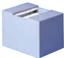
A hole is cut in the Soundblocker to accommodate the down lighter and the hood is simply positioned over this. The foam of the Soundblocker must not touch the fitting. The hood is manufactured from a non combustible material with 'Class 0' internal absorbent lining.
