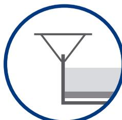
Soundblocker in a perforated spring tee tile, with foam facing downwards.
