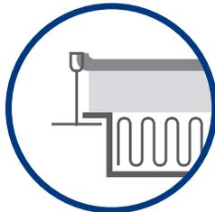
Lay in grid system with a metal tile, installed with a mineral wool pad. The Soundblocker is placed on top of the pad.
