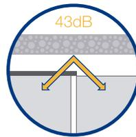
SoundBlocker installed in one room only ( $D_{ncw}$ )
